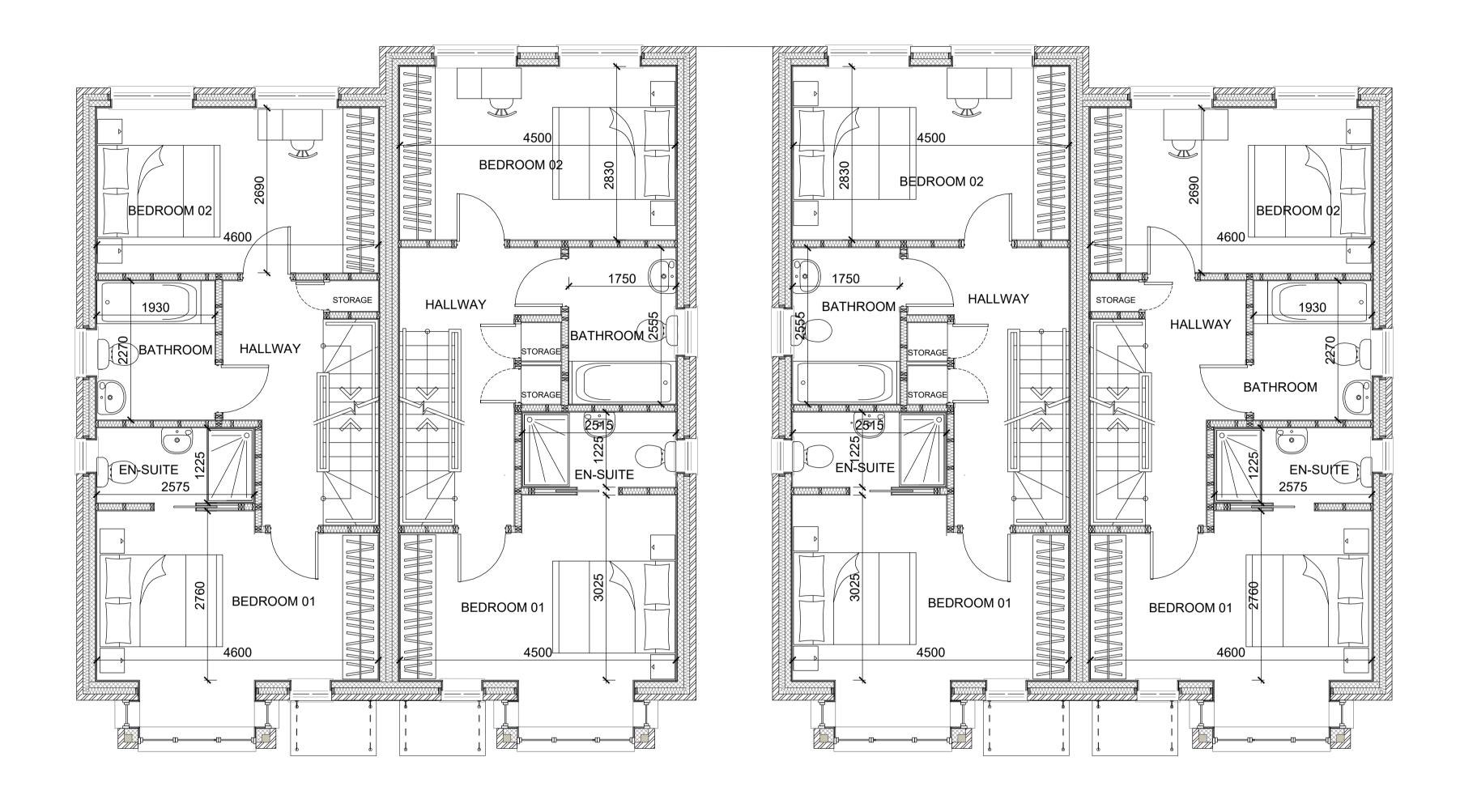
HOUSE 01, FIRST FLOOR GROSS INTERNAL AREA 44.40 M<sup>2</sup> HOUSE 02, FIRST FLOOR GROSS INTERNAL AREA
